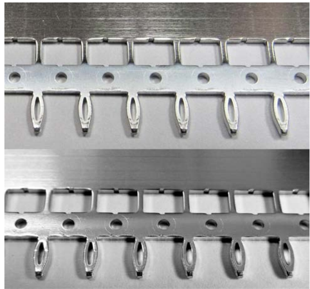
Techni Indium HS - Whisker resistant pure Indium plating deposit before and after reflow.
